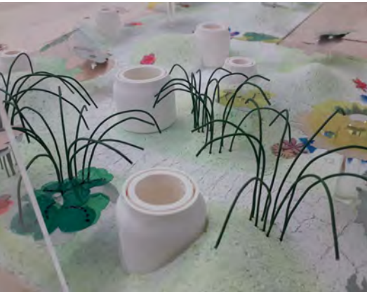
CNC routed polystyrene base with 3D printed buildings, L.Gerrard MArch thesis project: Andover Estate 2022
