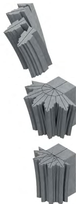
Exploded isometric – masonry blocks for vault ribs at Wells Cathedral Tracing the Past
